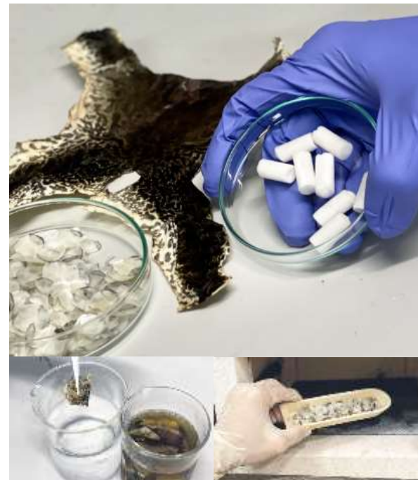
Collagen extraction from bullfrog skin, combined with HA (hydroxyapatite) from fish scales form the biomaterial a structure, composition that promote cell attachment PHOTO: NTU SINGAPORE
