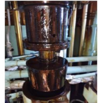
Excessive Filter Clogging Fuel Plunger Stuck in the Top Cover
