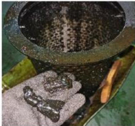
Hard Sludges from Filters, Pipelines, Purifiers
