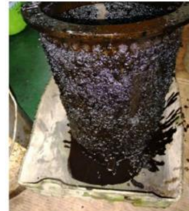
Excessive Filter Clogging Fuel Plunger Stuck in the Top Cover
