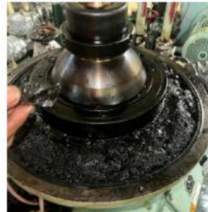
Hard Sludges from Filters, Pipelines, Purifiers
