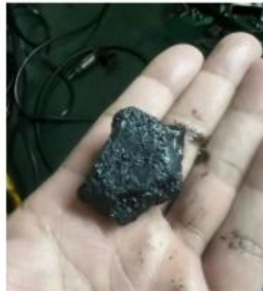
Hard Sludges from Filters, Pipelines, Purifiers
