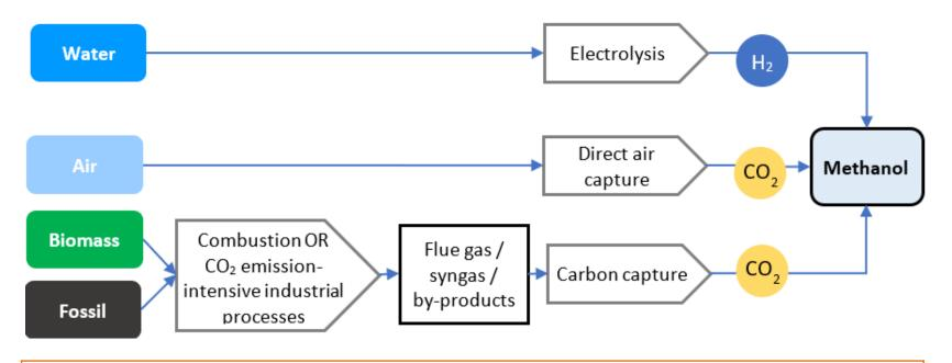
**Direct hydrogenation** of *pure* CO<sub>2</sub> and H<sub>2</sub> simplifies MeOH synthesis chemistry. Fewer reactions and by-products
