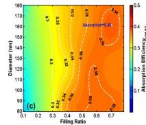
Highest light absorption exits in large volume filling ratio and a diameter of 162 nm
