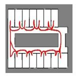
Goal oriented navigation in unknown environments must be able to adjust its existing plans based on the newly acquired environment data such as new obstacles and dead-ends. We have developed a new goal oriented navigation algorithm that is based on directing a robot's exploration towards the goal. It utilizes the SRFD approach's fast exploration data update rates to quickly detect and recover from dead-end situations and to send the robot in the correct
