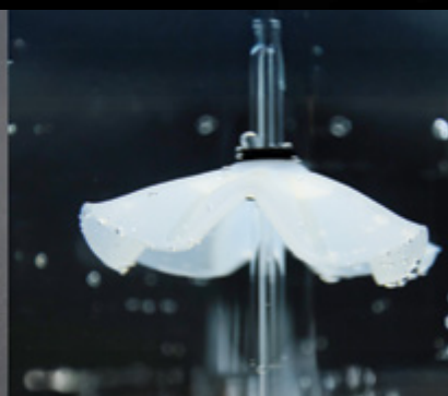
The umbrella device developed by the researchers closes when dry (left) and unfolds when wet (right). Credit: NTU.
