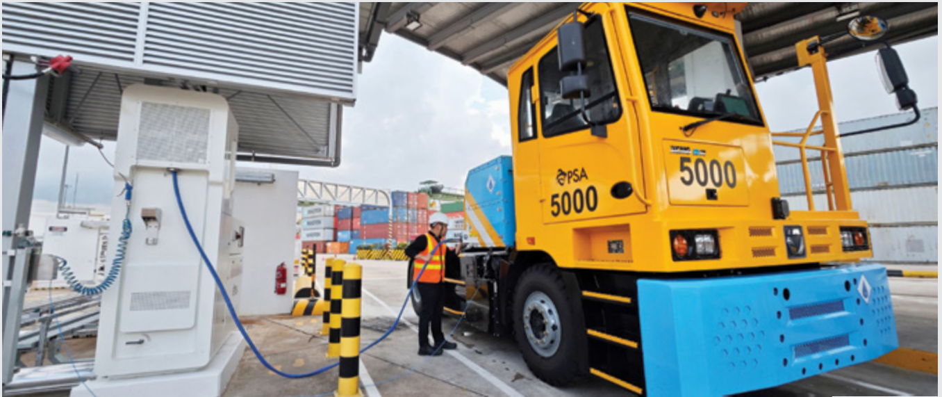
A hydrogen fuel cell-powered electric prime mover at PSA's hydrogen refuelling station. Credit: PSA Singapore.
