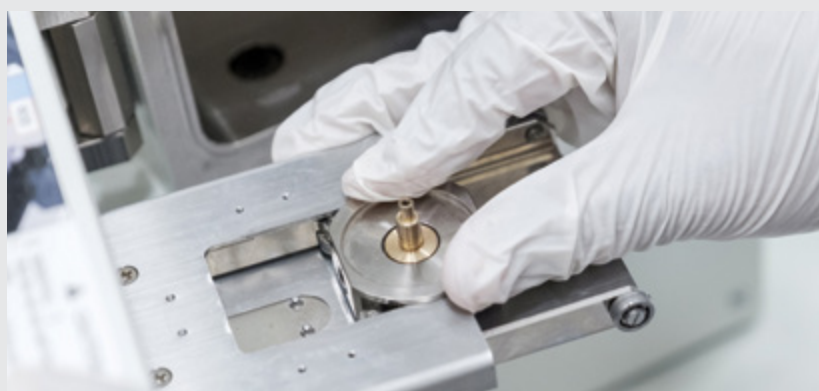
Graphite on a sample holder being loaded into a field emission scanning electron microscope for the NTU team’s X-ray experiments. Credit: NTU.
