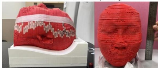
Modular design and assembly process for fabrication of phantom to preserve high degree of anatomical specificity to the individual patient
