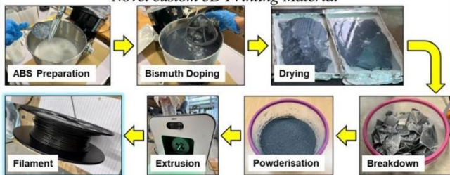
Novel custom 3D printing material was developed specifically to replicate the radiodensity characteristics of bone, achieving HU values otherwise unattainable with existing 3D printing materials
