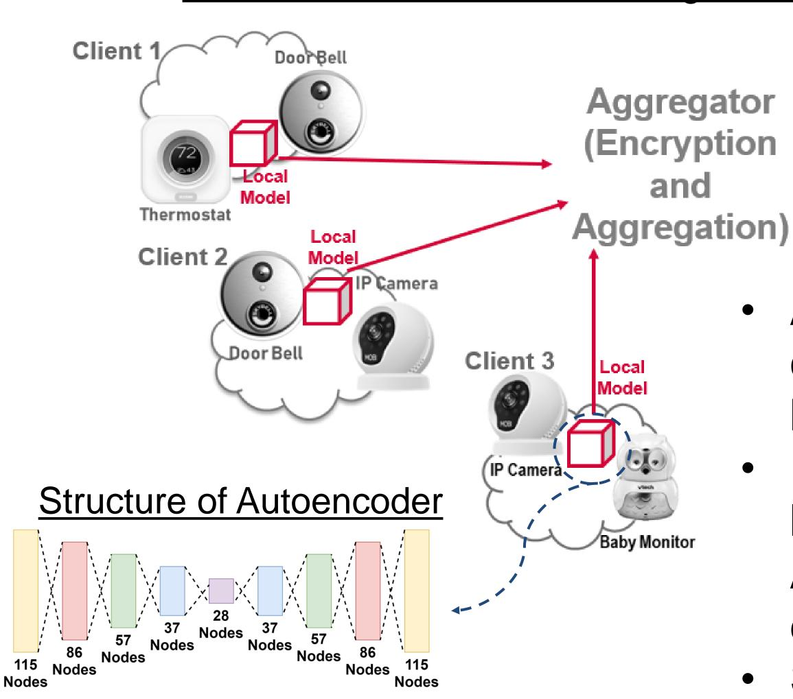
Allocate IoT devices to 3 clients to simulate 3 different home networks.
