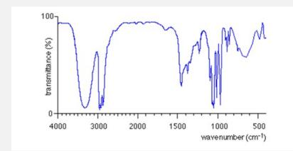
Fourier Transform Infrared Spectroscopy is an analytical technique used to identify organic, polymeric, and, in some cases, inorganic materials.
