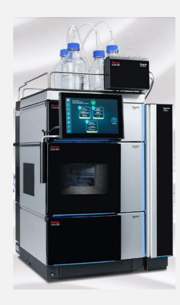
Ultra High Performance Liquid Chromatography (UHPLC) Ultra-high performance liquid chromatography (UHPLC) is a technique that separates the components of a mixture using high pressure.
