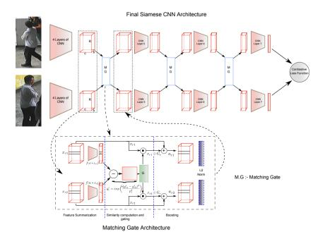
**Fig. 2. Proposed architecture:** The proposed architecture is a modified version of our baseline S-CNN proposed in Table 1. The matching gate is inserted between layers 4-5, 5-6 and 6-7. The detailed architecture of the gating function is also shown in the figure. See text for details. **Best viewed in color**
