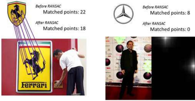
Fig. 12. There are two examples for the Ferrari and Mercedes logos, respectively. For the Ferrari logo (left), RANSAC works well since it has enough matched points to estimate the transformation model and does not constrain on the size of the objects; however, for the much smaller Mercedes logo (right), there are not enough matched points to estimate an accurate transformation model by RANSAC. On the contrary, the random partition method is less strict since it only assumes the target object appears in a compact local region. That means, when the target object is too larger than its assumption on object size, the random partition method may fail to accurately segment an entire object out. Instead, it tends to over-segment an entire object into a set of smaller regions. Therefore, compared to RANSAC, the proposed approaches are more competent for the small object search job.
