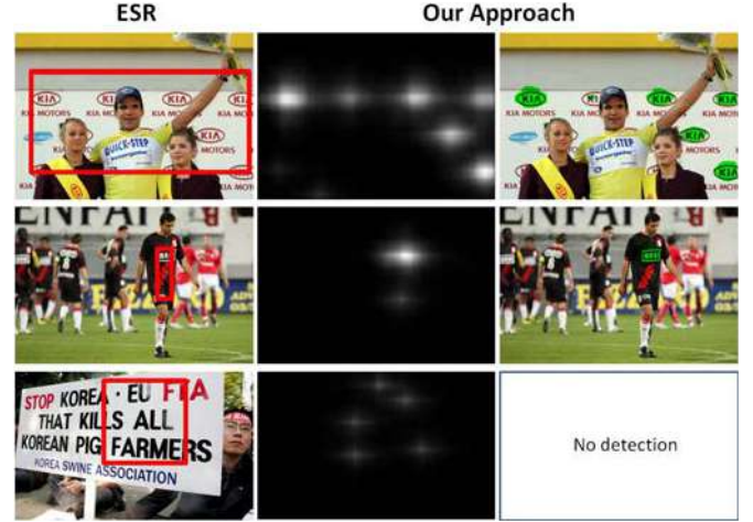
Fig. 13. Examples of the search results by ESR and our approach. The images in the first column are retrieved by ESR, in which the red bounding boxes are returned as the object location; the second column are the confidence maps generated by our NRP approach, and the third column are the segmentation results (highlighted in green). Note that each row stands for a specific case (from top to bottom): multiple target objects, noisy background and discrete matched points (false alarm by ESR).
