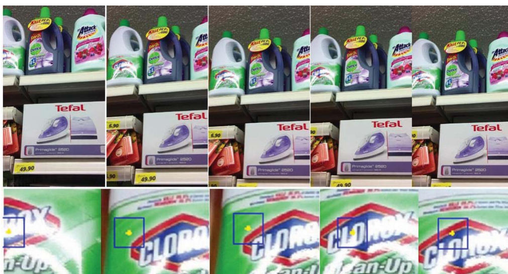
Fig. 3. Object detection with partial occlusions and reflections. The top row are the video key frames and the bottom row is the enlarged view of the detected locations of Clorox logo.
