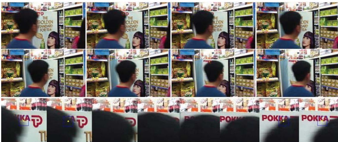
Fig. 1. Object detection with partial occlusions. The first two rows are video key frames and the third row is the enlarged view of the detected locations of Pokka logo.
